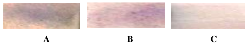
Figure 6. Stability sandwich-type optical immunosensor based on the alkaline phosphatase enzyme (A) 0, (B) 2 and 4 weeks
