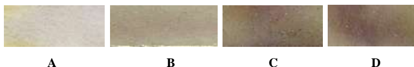
Figure 4. Color developed from 10^5 log CFU mL -1 Salmonella concentrations with different time incubation (A) 0, (B) 5, (C) 10 and (D) 15 minute.
