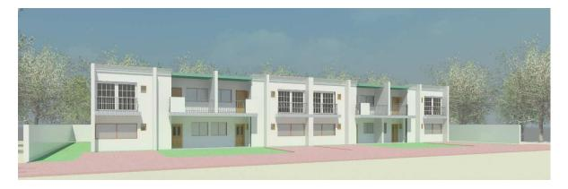
Building design for office use and radio station, consists of 3 levels of height, side warehouse and access to product discharge, steel design structure with masonry walls, was installed an elevator for personnel and cargo, in the roof space is left to swallow sunlight for better use of natural energy.
